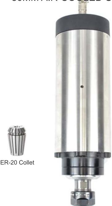
The optional 80mm Air-cooled spindle is virtually maintenance free. This spindle uses ER-20 collets, which can be purchased singularly or in both metric and imperial sets. The collet nut is ER20-A thread. The nut requires a 30mm wrench and the spindle shaft is held with a 21mm wrench. PROBOTIX sells collet sets and wrenches for these spindles. Be careful not to cross thread the nut.
