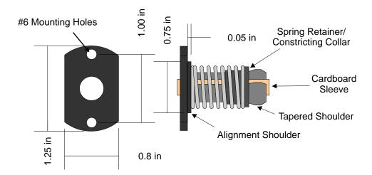
The anti-backlash nuts have a cardboard sleeve inserted in them that prevents the threads from compressing and allowing the spring retainer collar to slip over the tapered shoulder. Leave the cardboard sleeve in place and allow the screw to push it out as you thread in the acme screw.
