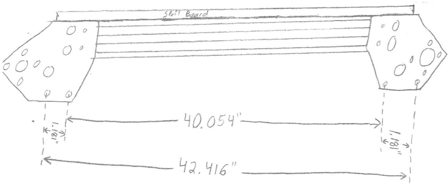
Spill Board is .750" thick
