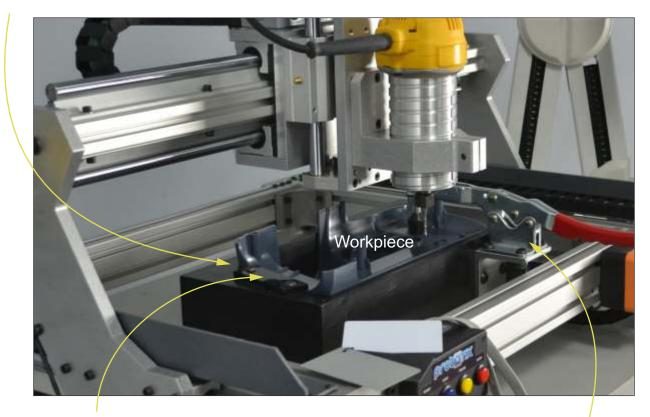
Negitive Shape Milled Into Delrin Block
