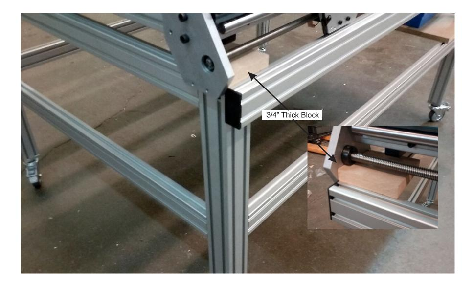
When you are ready to mount the machine to the machine frame, cut 3/4" thick blocks of wood to sit on top of leg. The drive screw shaft collars will sit on top of the blocks and give you perfect spacing. Don't be afraid to loosen any of the frame brackets to get the holes and slots in the feet to to line up - the frame doesn't need to be perfectly true.
