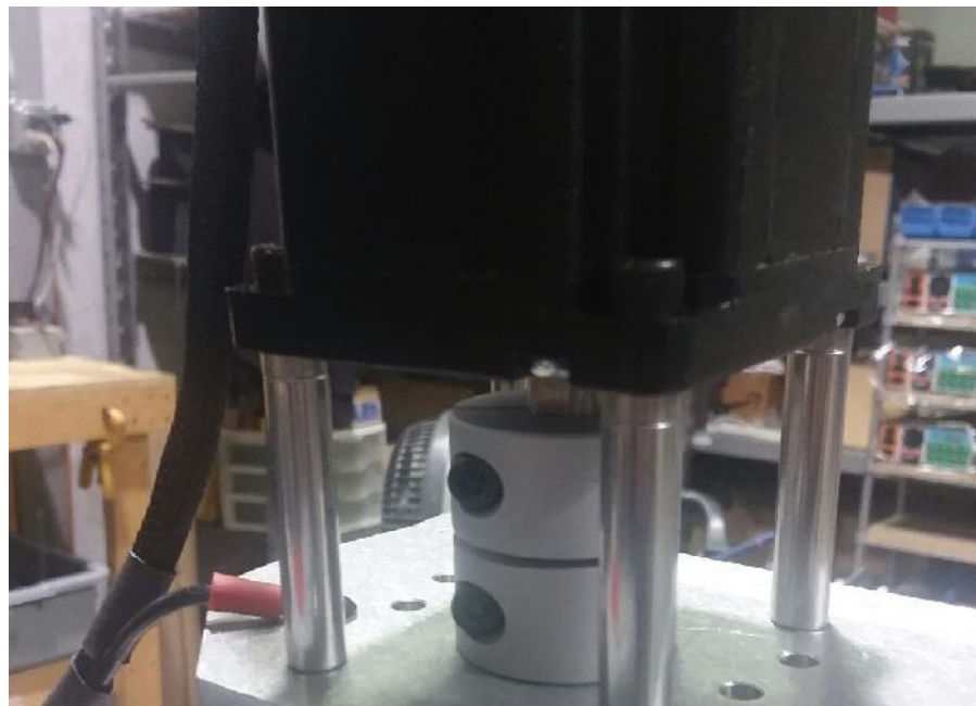
Finished Z Motor should look like above
