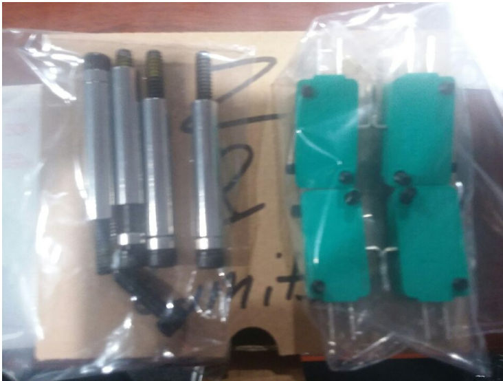
Box includes standoffs and limit switches shown
