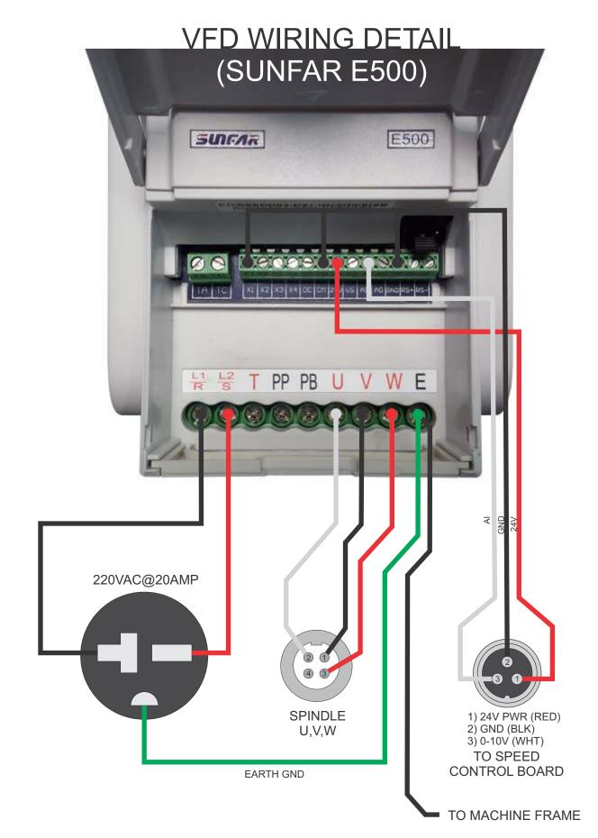
NOTICE: Internal wiring of Chinese spindles is not consistent. If spindle spins in reverse, swap U & V. You MUST verify visually or physically the proper rotation of the spindle to ensure the machine cuts properly!
