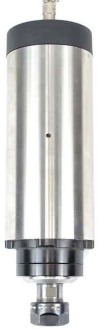
The optional 80mm Air-cooled spindle is virtually maintenance free. This spindle uses ER-20 collets, which can be purchased singularly or in both metric and imperial sets. The collet nut is ER20-A thread. The nut requires a 30mm wrench and the spindle shaft is held with a 21mm wrench. PROBOTIX sells collet sets and wrenches for these spindles. Be careful not to cross thread the nut.
