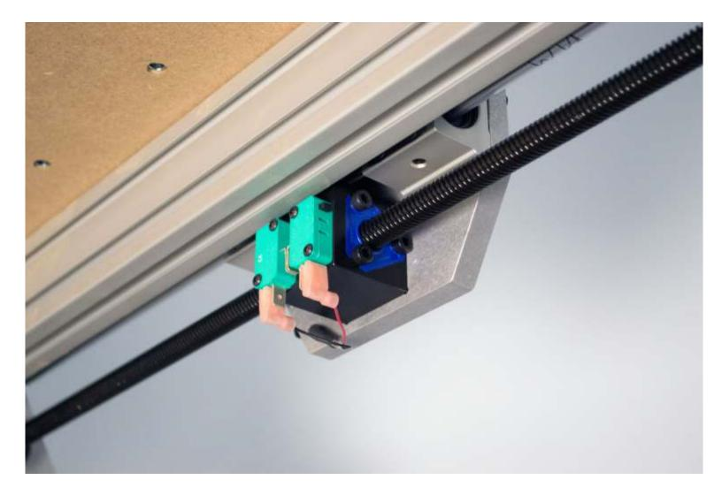
The Y1 and Y2 limit switches have been removed to protect them during transport. Reinstall them as seen above before running the machine.
