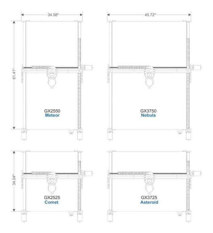
Machines should be placed on a level flat table, or mounted onto one of our machine stand kits. Refer to the diagram above for machine minimum table surface sizes. Felt pads can be placed under the machine's feet to dampen noise.
