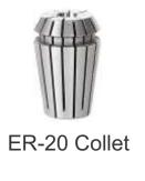
The optional 80mm Air-cooled spindle is virtually maintenance free. This spindle uses ER-20 collets, which can be purchased singularly or in both metric and imperial sets. The collet nut is ER20-A thread. The nut requires a 30mm wrench and the spindle shaft is held with a 21mm wrench. PROBOTIX sells collet sets and wrenches for these spindles. Be careful not to cross thread the nut.
